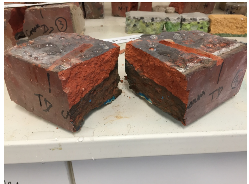
Breaking the brick from the centre of two injection holes: Cream has spread into the mortar joint & penetrated into the brick, forming a horizontal damp course.
