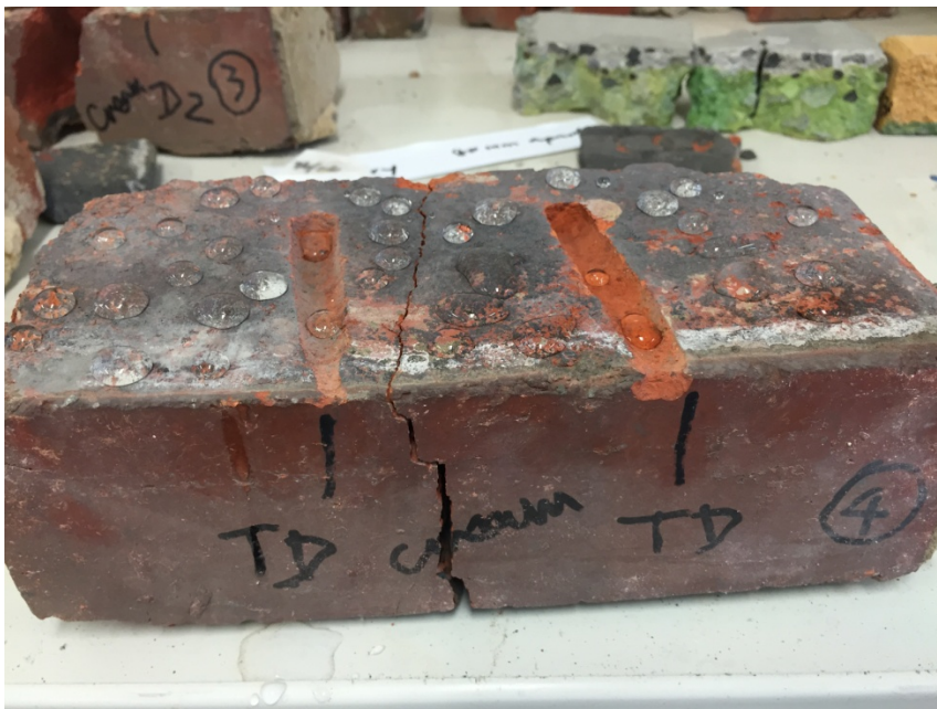
The whole brick surface and the mortar joint were water repellent
